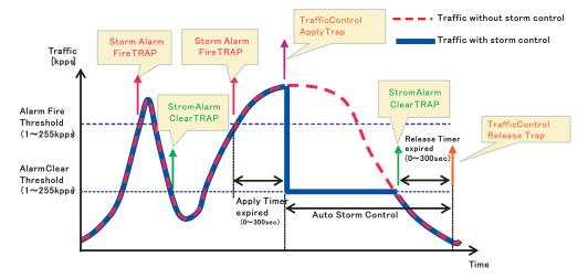
Figure 132: Storm Control by Limiting the Traffic Rate
