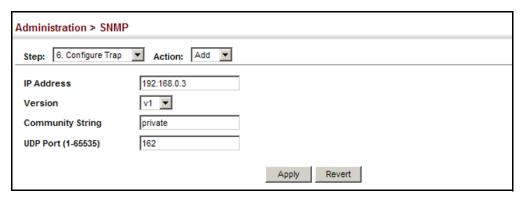
**Figure 274: Configuring Trap Managers** (SNMPv2c)
