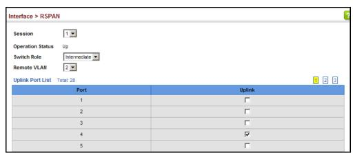
Figure 42: Configuring Remote Port Mirroring (Destination)
