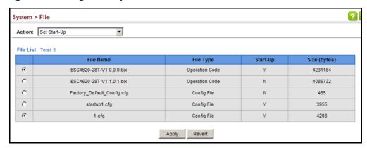
To start using the new firmware or configuration settings, reboot the system via the System > Reset menu.
