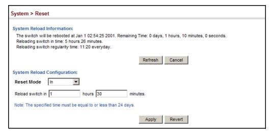
Figure 31: Restarting the Switch (At)
