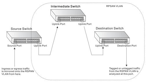
**Figure 39: Configuring Remote Port Mirroring**
