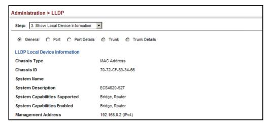
Figure 248: Displaying Local Device Information for LLDP (Port)
