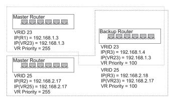
Figure 458: Several Virtual Master Routers Configured for Mutual Backup and Load Sharing
