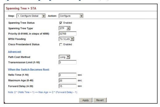
Figure 115: Configuring Global Settings for STA (RSTP)
