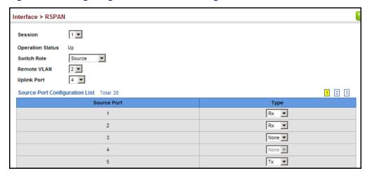
Figure 41: Configuring Remote Port Mirroring (Intermediate)
