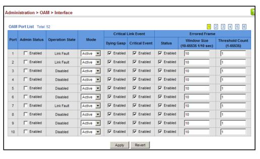
**Figure 330: Enabling OAM for Local Ports**
