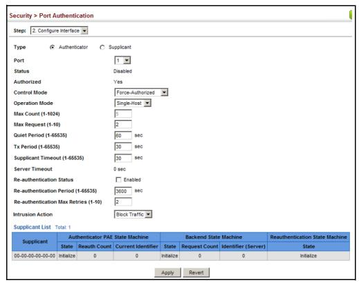
Figure 222: Configuring Interface Settings for 802.1X Port Authenticator
