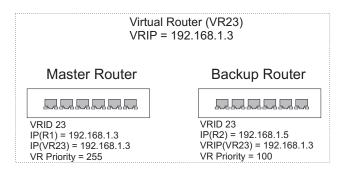
Figure 457: Several Virtual Master Routers Using Backup Routers
