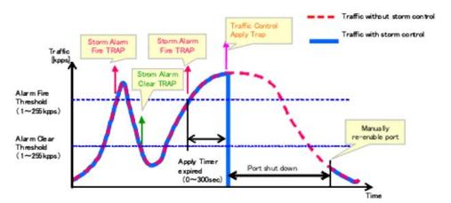
Figure 133: Storm Control by Shutting Down a Port
