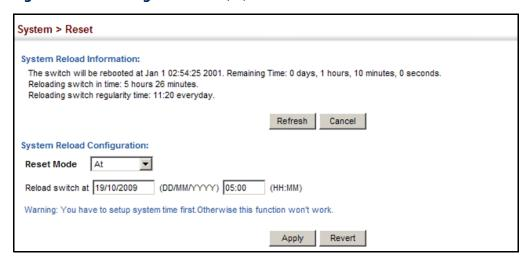
Figure 32: Restarting the Switch (Regularly)
