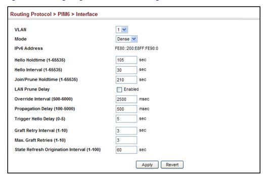
Figure 538: Configuring PIMv6 Interface Settings (Sparse Mode)
