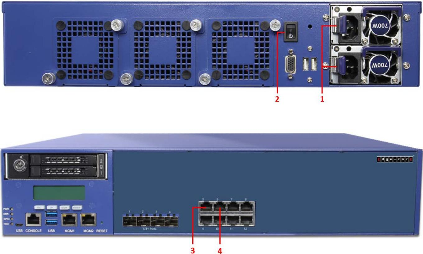
1. Connect the power cord to the power socket on the rear panel.
