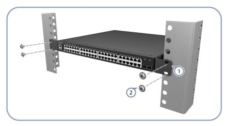
1 Attach the brackets to the switch.
