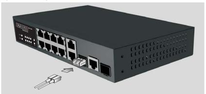
**4.** As a connection is made, check the Link LED on the switch corresponding to the port to be sure that the connection is valid.
