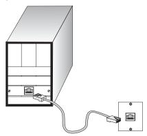
2. If the device is a network card and the switch is in the wiring closet, attach the other end of the cable segment to a modular wall outlet that is connected to the wiring closet. (See the section "Fiber Optic SFP Devices.") Otherwise, attach the other end to an available port on the switch.
