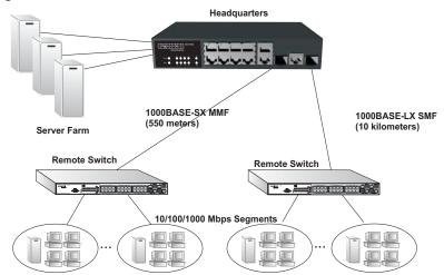
Figure 7: Remote Connections with Fiber Cable
