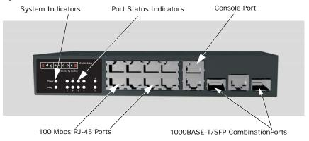
If an SFP transceiver is plugged in, the corresponding RJ-45 port is disabled for ports 9-10.
