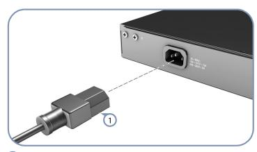
1 Plug the AC power cord into the socket on the rear of the switch.
