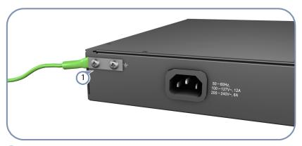
Onnect a grounding wire and lug to the dual-hole grounding point on the switch rear panel, then to rack ground.
