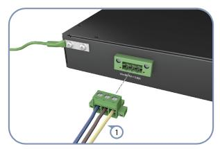
(1) Plug the DC power cable into the socket on the rear of the switch.
