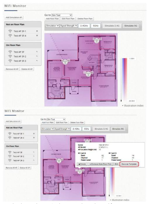
Configurations can then be saved conveniently to a template to be used for AP Management.
