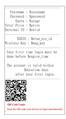
On-Demand Account generation with a ticket generator is a very common deployment for hotspot providers. What makes it a hassle is to manually enter the Username and Password of the account, especially for mobile devices which require typing on small keyboards and are not easy on the eyes.
