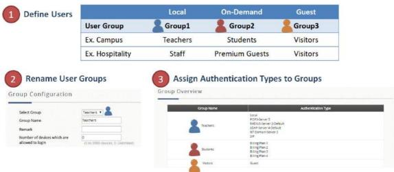
In the WLAN controllers, there are eight to twenty-four Group profiles, depending on the model capacity. Besides, the system does provide several flexibilities for mapping from different authentication options
