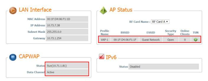
5. On AP: to reconfirm the specific VAP Configuration is under Complete Tunnel
