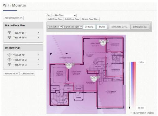
Click "Simulate 2.4G" or "Simulate 5G" to see if the deployed APs are adequate for your requirement.
