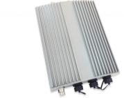
Edgecore ECWO5210-L is an enterprise-grade, concurrent dual-band 802.11ac outdoor access point, designed specifically to withstand harsh weather conditions in outdoor and industrial environments.
